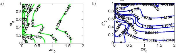
Fig. 6. Electric field effect on development of axial (a) and radial (b) velocity profiles downstream combustor at  $P_e = 0.5$
