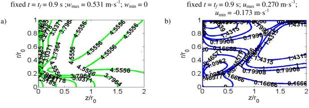
Fig. 7. Electric field effect on development of axial (a) and radial (b) velocity profiles downstream combustor at  $P_e = 1.0$
