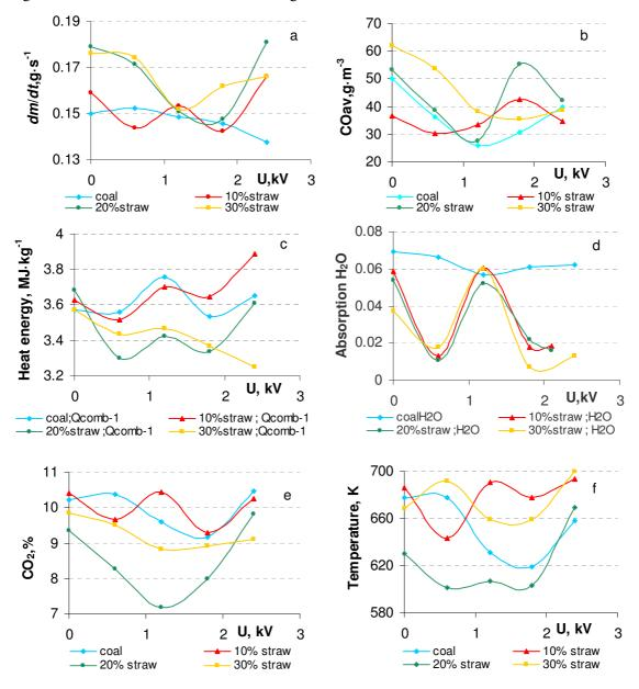
Fig. 8. Electric field-induced variations of weight loss rate (a), density of volatiles entering the combustor (b), produced heat energy in the flame reaction zone (c), H<sub>2</sub>O absorption (d), CO<sub>2</sub> volume fraction (e) and products temperature (f)
