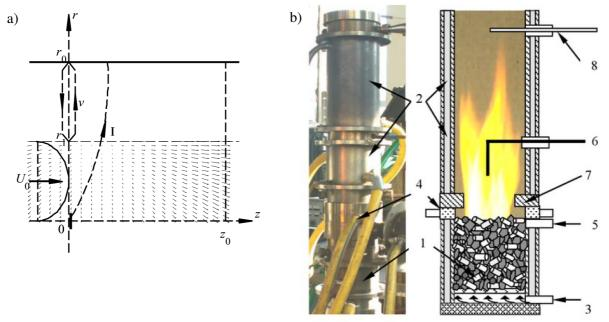
Fig. 1. Digital image of computational domain (a) and schematic of experimental device (b):
